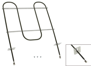
UT306 (2400W/240V) Broil Element 13"W x 14" L x 3-7/8" insert
