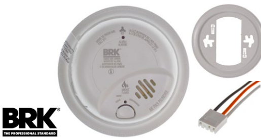
BRK Hardwire Ionization Smoke & Carbon Monoxide Alarm, 9V Battery Backup, 120V AC 60Hz - Part # SC9120BA
